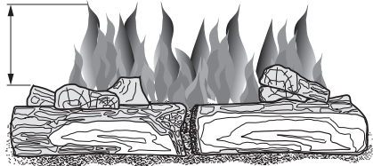
Figure 22 - Incorrect Burner Flame Pattern
