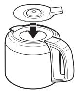
2. Rotate the lid counterclockwise until the thumb lever is over the handle.
