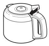
3. To pour, press the thumb lever down.
