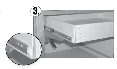
Start a screw at the endpoint of the slide. Continue to add screws and then pull the drawer box out further to finish the process. Remove brackets and you have perfect drawer box alignment!
