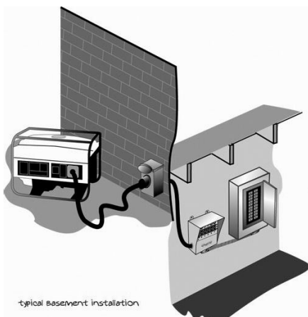
Generator Plugged into Outdoor Power Inlet Box Wired to Transfer Switch Next to Basement Load Center (POSSIBLE KIT INSTALLATION)
