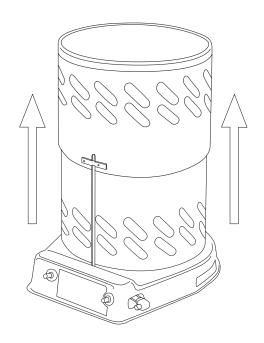
STEP 2: LIFT OUTER SHELL STRAIGHT UP. CARE MUST BE TAKEN TO PROTECT HANDS DURING LIFT.
