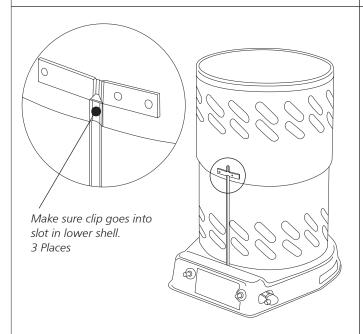
STEP 3: LIFT OUTER SHELL UNTIL ALL THREE CLIPS ENGAGE SLOTS IN LOWER SHELL. WHEN THIS HAPPENS, THE SCREW HOLES WILL LINE UP.
