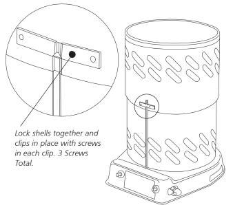
STEP 4: LOCK THE CLIP INTO PLACE WITH 3 SCREWS AS SHOWN. THE HEATER MUST NOT BE OPERATED UNLESS THE OUTER SHELL IS PROPERLY EXTENDED AND FULLY LOCKED INTO PLACE.
