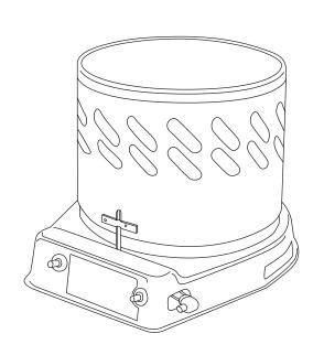
STEP 1: HEATER AS RECEIVED OUT OF BOX. BEFORE LIFTING OUTER SHELL PROTECT HANDS. NEVER GRASP BARE METAL WITHOUT HAND PROTECTION.
