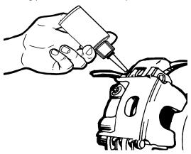
Any excess grease that squeezes out from the mating surfaces should be removed.
