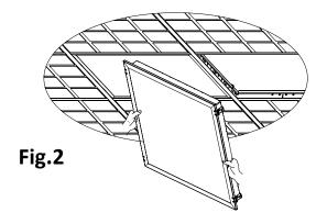
Insert the troffer into the ceiling grid, attach the earthquake clips to the ceiling grid. (Fig.3)
