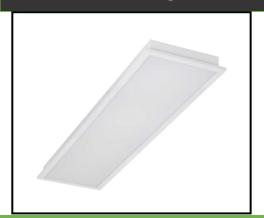
The ETi Backlit LED Recessed Troffer offer a slim, low profile and easy to mount design. The luminaire provides for a brighter, lighter weight and more efficient replacement for standard fluorescent lay-in troffer used in recessed ceiling lights. Fixture is supplied with a 100-277v driver. Warranty period 5 years or 60 months. Suitable for installations from – 4° F to 104° F.
