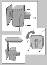
**Vehicle Alert Installation:** For cars, the best mounting position is about 4 feet (1.2 m) high, between 10-20 feet (3-6 m)back, and angled to see the back of car after passing the sensor.
