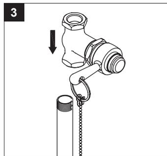
4. Attach water distribution pipe and shower arm (not included) to shower valve. Make sure distribution pipe is properly supported.
