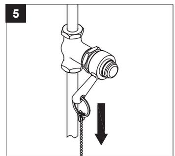
6. Release chain, water should shut off. Check for leaks.
