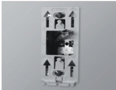
5. Take the wires from the wall through the hole at the base of the mounting base and connect them using the supplied solderless connectors. When making the connection with aluminum wire, make sure that you are using connectors identified CO/ALR. Please note that the thermostat wires do not have polarity. Therefore, the way they are connected is not important.
