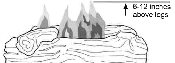
Fig. 30 - Incorrect/Abnormal Flame Pattern with tall flames
