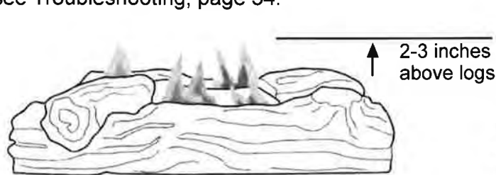
Fig. 22 - Correct Burner Flame Pattern
