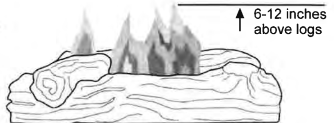
Fig. 23 - Incorrect Burner Flame Pattern
