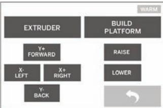
The screenshot shows the printer's control panel with the 'WARM' indicator. The main display area is divided into two sections: 'EXTRUDER' and 'BUILD PLATFORM'. Under 'EXTRUDER', there are buttons for 'Y+ FORWARD', 'X- LEFT', 'X+ RIGHT', and 'Y- BACK'. Under 'BUILD PLATFORM', there are buttons for 'RAISE', 'LOWER', and a 'BACK' button (curved arrow icon).
