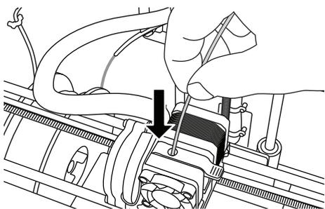
**⚠ WARNING** Do not touch the extruder tip during Dremel 3D20 operation or until it has cooled down to at least 60°C (140°F). Contact with the extruder tip during or after operation before tip has cooled may result in personal injury.
