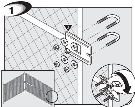
Fully open gate. Attach gate stop plate on the inside of the gate with one of the following:
