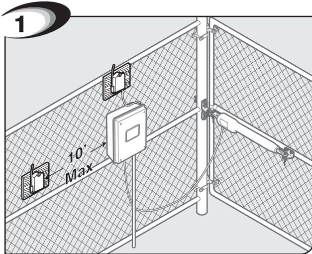
Install Receiver within 10 ft of control box (longer lengths available - call us). **NOTE: NEVER splice receiver cable. DO NOT run cable through metal conduit because the receiver signal range will decrease. DO NOT run cable through conduit containing AC wire. DO NOT place receiver within 3 feet of AC power.**
