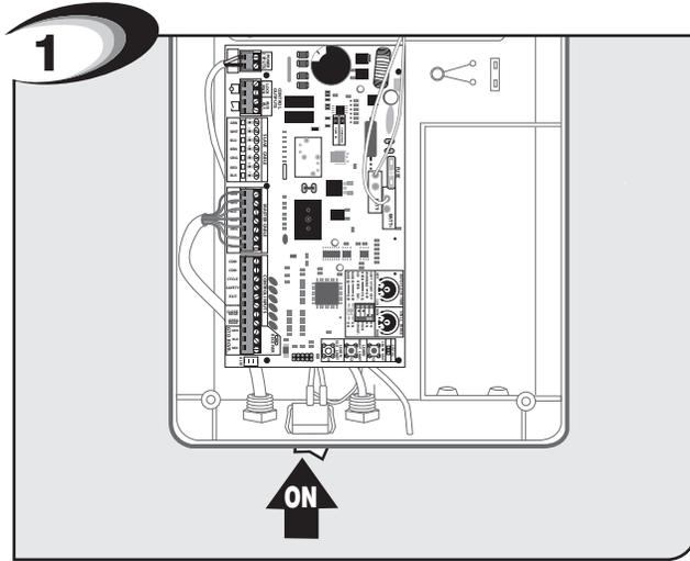
With gate in CLOSED position, turn control box power switch to ON.
