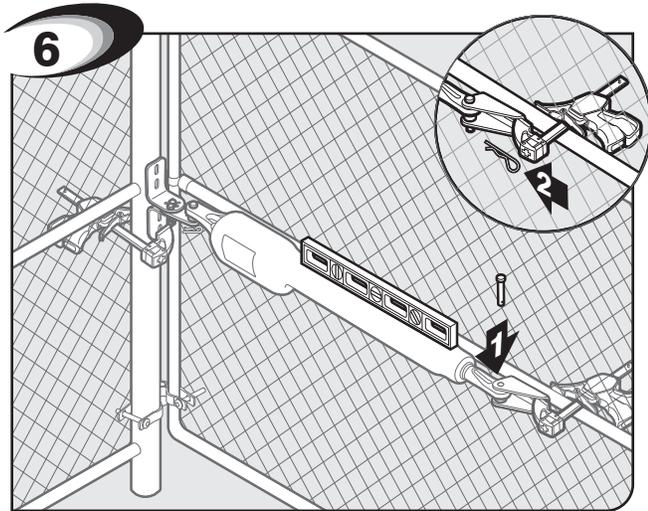
6 OPEN gate and re-attach opener with clevis pin. Check for level. Clamp securely.
