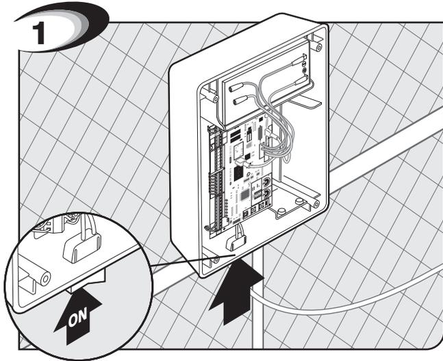
With gate in OPEN position, turn control box power ON.
