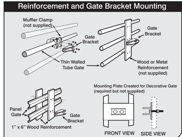
Recommended reinforcement and gate bracket mounting examples (muffler clamp does not require drilling and is adjustable).
