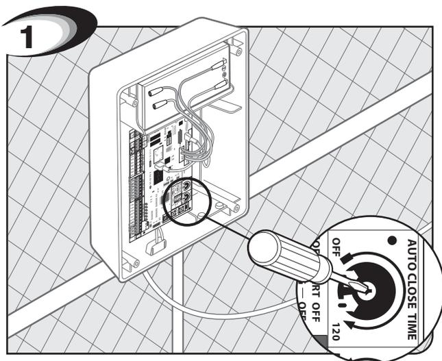
Turn the “AUTO CLOSE TIME” arrow in the center of the potentiometer with small flat head screwdriver. Turning the pot all the way counter-clockwise will turn the auto close feature off. The minimum auto close time is 3 seconds. The maximum (turn the pot all the way clockwise) auto close time is 120 seconds.
