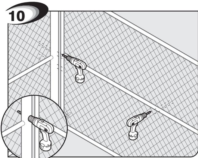
10 Drill 3/8" holes completely through gate post and gate cross support.
