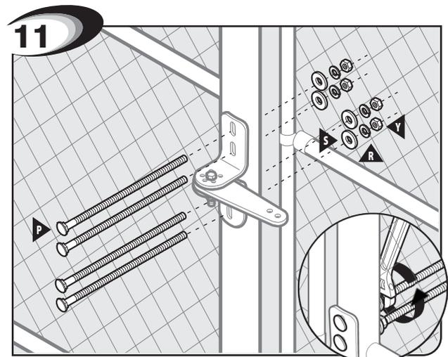
Attach post bracket assembly to fence post. **NOTE:** Must be through bolted.
