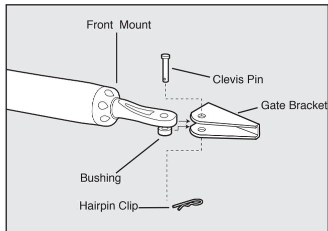
**NOTE:** Substitute a **Pin Lock** for the clevis pin on the front mount of the gate operator to prevent theft of the operator from the gate (*see accessory pages in back of this book*).
