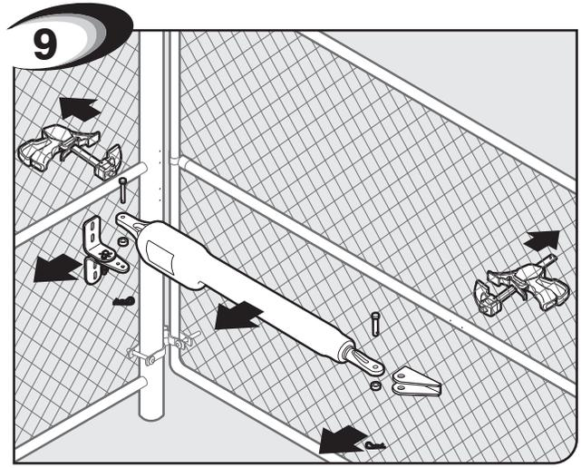
9 Remove clamps, post, gate brackets, and opener. Then use a hammer and center punch to dimple hole positions for drilling.
