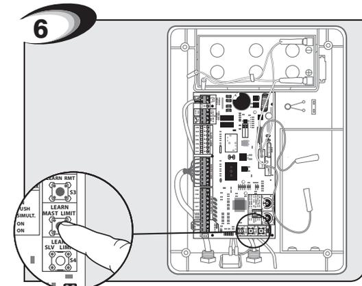
Hold the "LEARN MASTER LIMIT" button for 10 seconds, or until the alarm sounds to clear. Go back to setting open gate limit step 1 at the top of this page.
