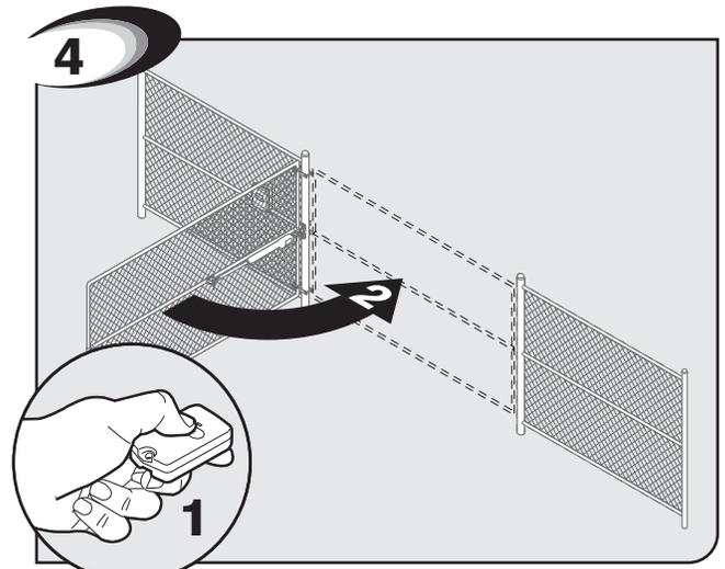
Press button on opener remote to fully close gate. Open limit is set upon reaching the fully closed limit. Test and, if needed reset and start over.
