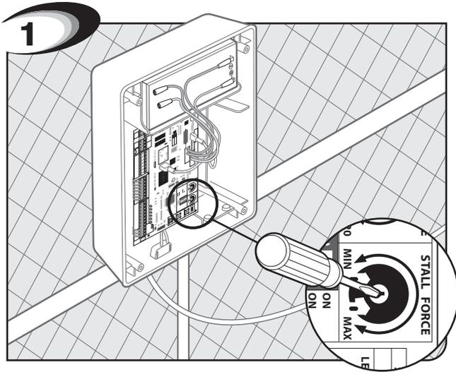
Do not use the Dual Sense Stall Force adjustment to compensate for a gate that is sticking or binding. Excessive Stall Force may cause damage to the gate operator or gate system or Injury or Death.
