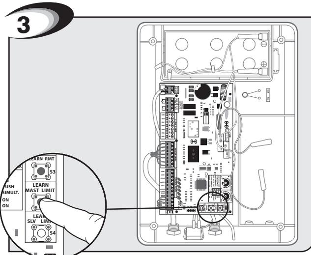
Press and hold the "LEARN MASTER LIMIT" button for 5 seconds, or until the alarm sounds.
