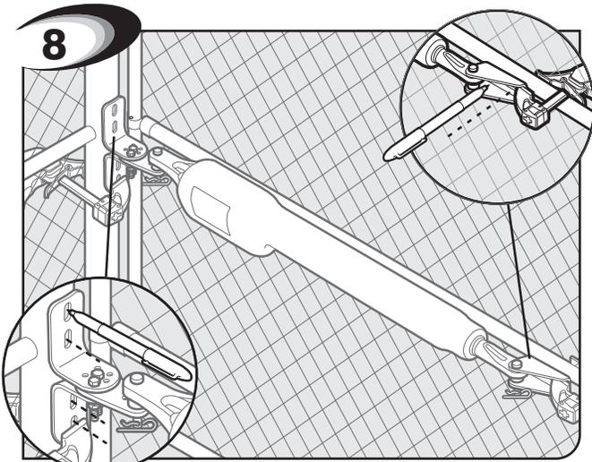
8 Mark middle of post bracket slots on fence post. Mark middle of gate bracket slots on gate cross support.
