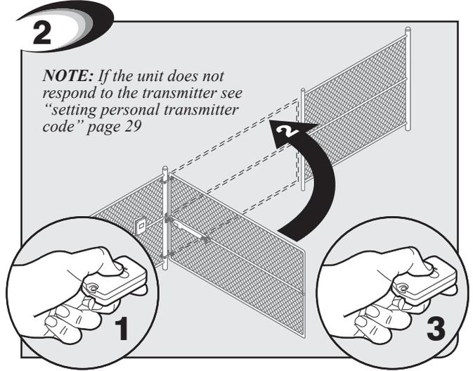
Press button on opener remote; gate should start closing. Press button on opener remote again when gate is in desired CLOSED position.
