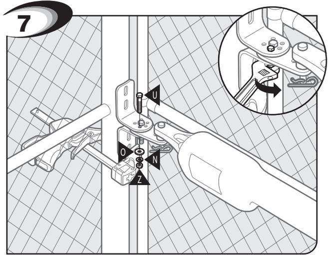
7 Secure post pivot bracket to post bracket when clearances are OK (Step 5) in both open and closed positions.
