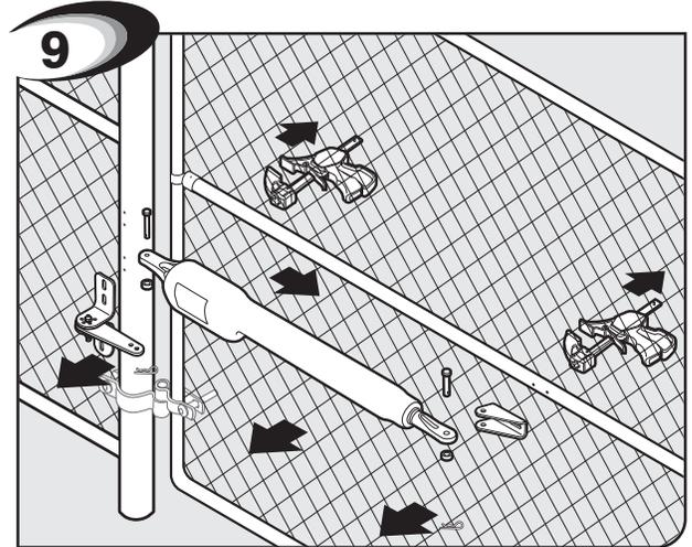
Remove clamps, post, gate brackets, and opener. Then use a hammer and center punch to dimple the hole positions for drilling.
