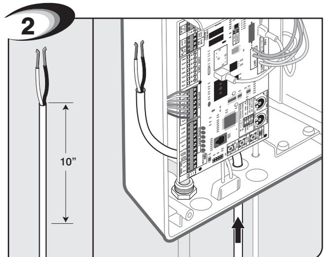
Feed 10" of wire from solar panel into box through the pre-drilled hole in the bottom of the control box.
