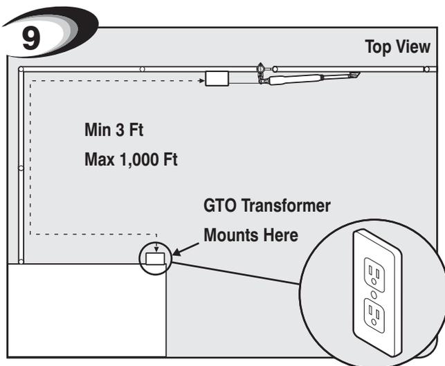
Locate power outlet and identify wire path to control box.
