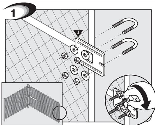
Fully open gate. **On push-to-open gates attach gate stop on the outside of the gate with one of the following:**
