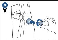
Place extension wand clip on back of unit, twist clockwise to lock in.
