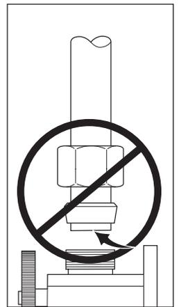
Ensure tube is fully inserted into stop before sliding sleeve down to engage top of fitting.
