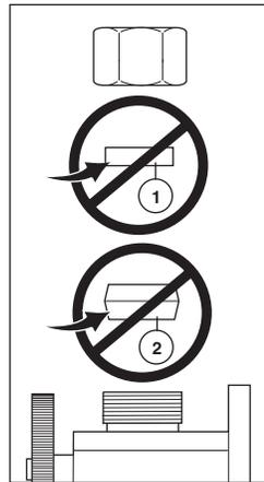
Do not use RP51243 gasket (1) supplied with PEX tubing or brass ferrule (2) supplied with valve stops.
