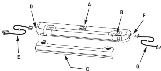
**3** Mount 1st unit using the two wood screws provided. Plug the Power Input Cord into Power Input Connector as shown in Fig. 1. This connector is designed to go into only one end of the lamp. If it cannot be latched in place, try the cord on the other end of the lamp. Do not force the plug into the socket.
