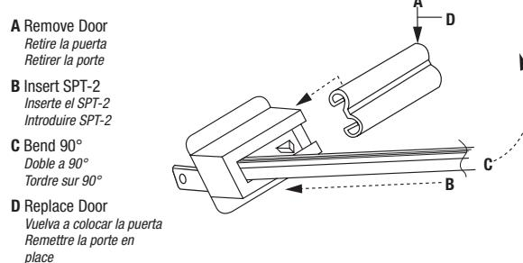
**Note: VERY IMPORTANT!** The ribbed side of the SPT-2 cord (common), must pierce with the ground prong contact (see fig.3).
