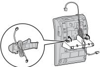
4 Drive screws (not included) into the wall using the wall template below. Connect the telephone line cord. Mount the unit, and then slide it down.
