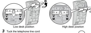
J Tuck the telephone line cord inside the wall mount adaptor, and push it in the direction of the arrow.
