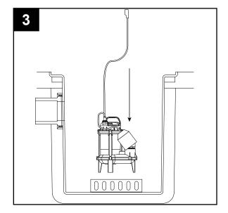
4. Place the pump inside the basin with the switch positioned away from incoming water.
