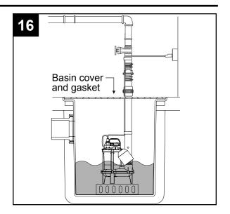
17. Install a vent pipe (not included) according to local, regional, or state codes to remove gases and odors.
