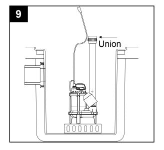
10. Install a 2 in. check valve (not included) above the union to prevent back-flow.
