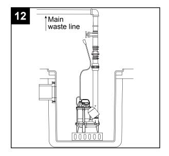
13. Attach power supply cord to discharge pipe using cable or zip ties (not included) to allow the float switch to move freely.
