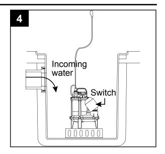
5. Be sure the float switch is at least 1 in. away from the side walls of the basin and free of any obstructions through the full range of switch motion.
