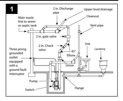
2. These pumps are equipped with a float switch. The pump will turn on automatically when the water level in the basin reaches the "on" level.
