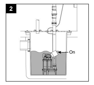
3. The pump will turn off automatically when the water level in the basin reaches the "off" level.
