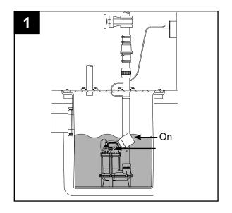
2. Remove any debris from the basin that could interfere with the operation of the switch.
