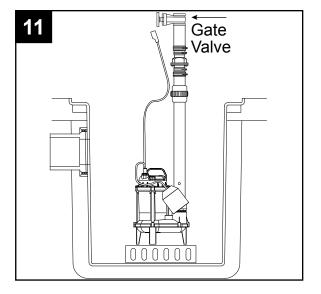
12. Connect remaining discharge pipe into main waste line to sewer or septic tank.
