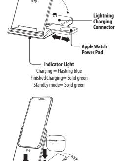
Place wireless charging enabled device on the Power Pad to begin charging. Place earbud case on to the lighting charging connector.
