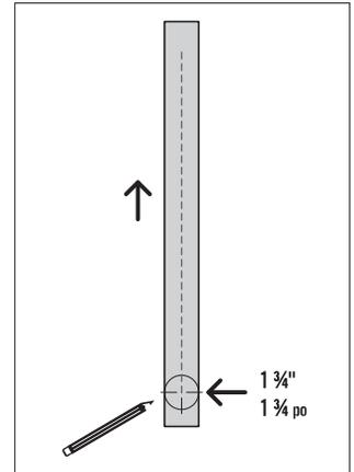
2. Mark  $3 \frac{1}{2}$ " on the post from the bottom of the opening, centered on the previous line from Step 1.
