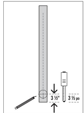
3. Using one of the actuators provided, place it with the bottom circular hole on top of the  $3 \frac{1}{2}$ " marking from Step 2. Mark the next spot using the second circular hole above in the actuator. Continue this until you reach the top of the opening.
