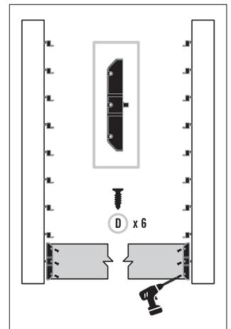
6. Attach each actuator one at a time, to either the left or right side. Connect each one to the next bracket using Screw C, overlapping it onto the next - there is an indent, so they will be flush when you connect them.
