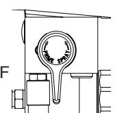
4. Move the PRIME/SPRAY valve down to the PRIME position.
