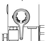
6. Set the pressure to Turbo RAPID CLEAN by turning the pressure control knob to its RAPID CLEAN position.
