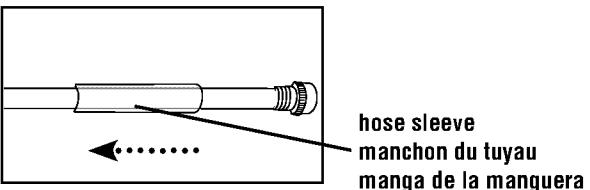
**IMPORTANT INSTRUCTIONS:** When attaching the garden hose to the hose reel out-tube, be sure to attach correctly (Fig. 1). Cross-threading could cause permanent damage.
