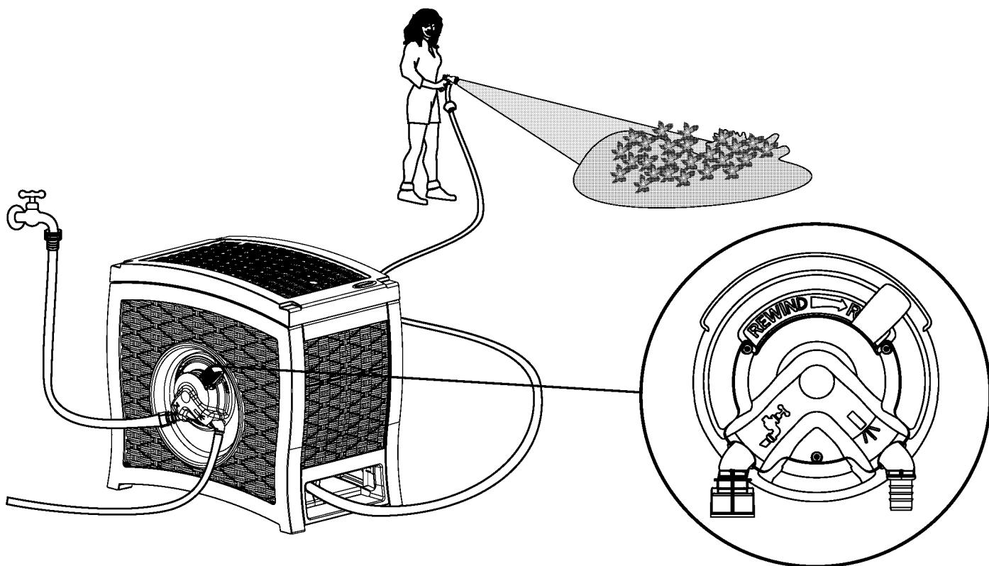
To unwind hose, position the lever at the side of the unit on REST mode, and pull hose out of unit. Turn on water source and use.
