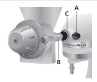
Tighten the attachment knob (A) until the unit is completely secured to the mixer.
