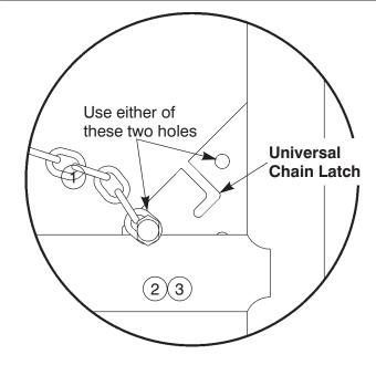
**NOTE:** For the safety of your horse, make sure the nut is located to the outside of the enclosure.
