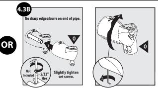
Some models may feature a slip fit installation with no threaded adapter in the tub spout. For these installations, slip the tub spout onto pipe pointing up and slightly tighten the set screw. Rotate tub spout to final position and fully tighten set screw in place.
