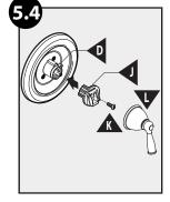
After setting the adjustable temperature limit stop to the desired position, remove the lever (L), reattach the lever handle adapter (J), adapter screw (K), and lever (L) – make sure ridges on back of (J) are to the left of the tab on (D).
