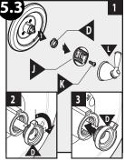
Remove the lever (L) and lever handle adapter (J). Note the position of the stop. Position the adjustable temperature limit stop (D) so the lever tops at that position. This prevents the lever from being turned into an unsafe temperature.
