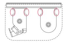
Using provided fasteners, mount the rope cleat to the wall to store excess rope. When a ladder is up on a ceiling, the excess rope should be stored on the cleat.
