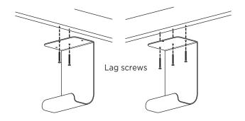
Measure the distance between the outermost rungs on the ladder to mark the two hanging points. Mark the distance on your ceiling from the center of the J-hook to the center of pulley assembly.
