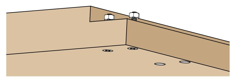
If you are using flat head bolts, you must first counter-sink the underside of each hole, and then insert the bolt up through the bottom of each hole. With the bold protruding from the top side of the hole, begin to thread a ¼" nut onto it until the bolt begins to protrude form the other side.
