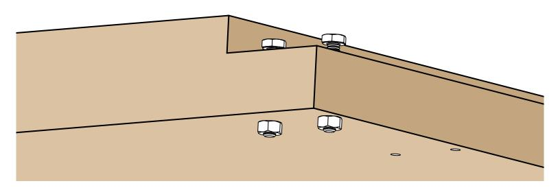
If you are using hex head bolts, insert the bolts down through the top of each hole and thread the nuts until the bolt begins to protrude from the other side.
